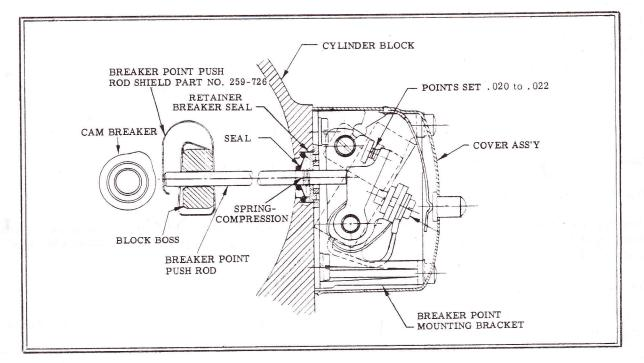
INSTALLATION OF 259-726 Breaker Point Push Rod Shield
