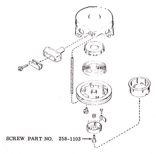
On older model engines using the above Recoil Starters center screw part no. 258-1103 was a #10-32 thread. Later model engines with the above Recoils will be using a screw with a #12-28 thread.
