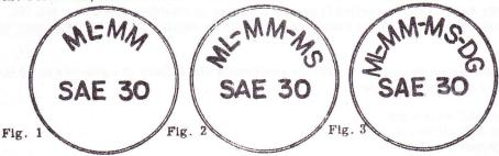
SERVICE ML - This is a service typical of gasoline engines used under light and favorable operating conditions. It includes moderate speed or moderate load operation most of the time with no severe low or high engine termperature operations. NOTE: NOT acceptable in a Clinton 4-cycle engine and use of ML rated oil voids engine warranty.
